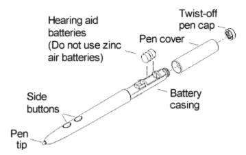
**Note:** When you replace the pen batteries, the pen will reset to the default frequency. If you changed the frequency of the pen before replacing the batteries, you will need to do so again after replacing the batteries (see the Reducing Monitor Interference section in Solving Problems).
